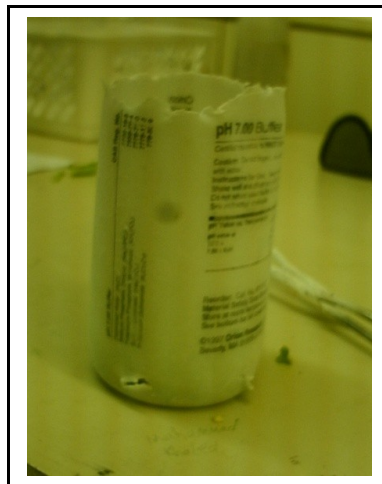
Figure 3.6: Plastic container used for treating pepper samples with liquid nitrogen for further analysis in the future.
