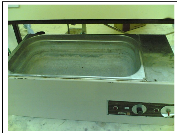
Figure 3.1: Temperature-controlled water bath used for treating pepper fruits by hot water dipping in different temperature and time.
